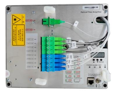
Note: The optical signal of the downstream network is amplified and transmitted in the FTTX network. One channel of input CATV 1550nm signal, eight channels of input OLT PON 1490nm signal, and eight channels of output combined optical signal ports are connected to the user terminal ONU through the ODN network respectively.
